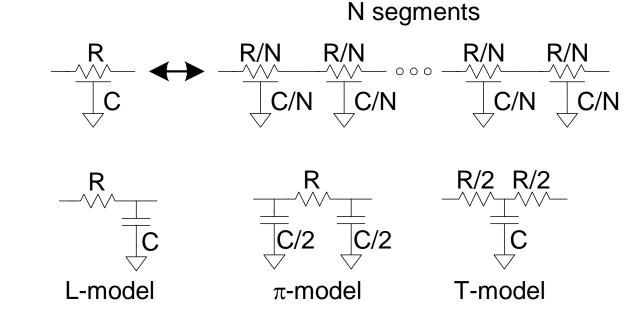
3 segment  $\pi$ -model is accurate to within 3% in simulations
