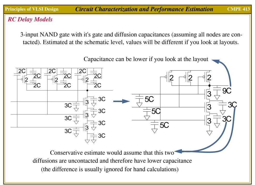
**Circuit Characterization and Performance Estimation Principles of VLSI Design CMPE 413 RC Delay Models: Layouts** Good layout minimizes diffusion area. NAND3 gate shown below, shares one diffusion contact, thus lowering the output capacitance by 2C. Contacted diffusions are assumed. vdd 2CShared Contacted Diffusion Isolated Contacted 2 2 Merged Diffusion Uncontacted Diffusion 3C 3C and 3C 3C 3C
