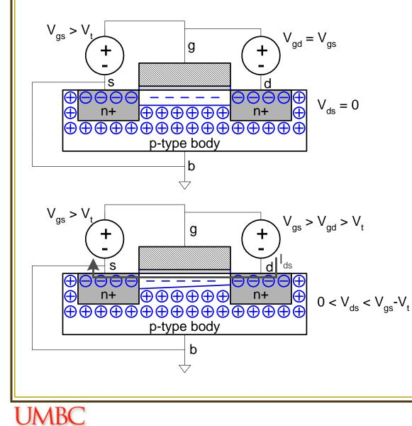
Channel is formed and extends from the source to the drain
