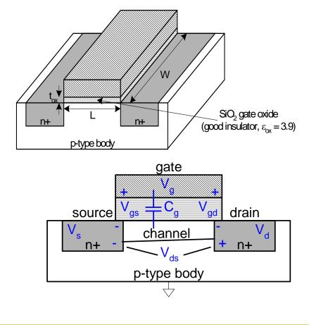
MOS structure looks like parallel plate capacitor while operating in inversion (*Gate-Oxide-channel*)
