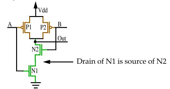
The source-to-substrate  $(V_{sb})$  may increase at this connections
