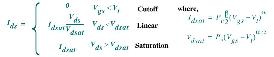
where the parameters,  $\beta P_c$ ,  $\alpha$  and  $P_{\upsilon}$  are obtained by curve-fitting the I-V characteristics.
